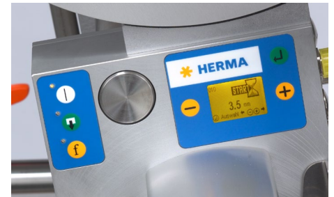
Clearly-defined display panel facilitates adjustments to operational parameters; provides 30 preset functions
